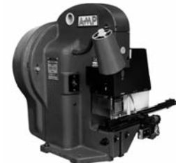
AMP-O-LECTRIC Bench Machine with Special Applicator
